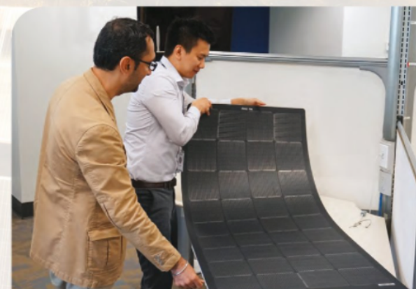
(L to R) Senior Marketing Manager Mitul Chandrani and Product Manager Wesley Shuen inspect a Solar Max solar panel. The product team developed the flexible panel that can be rolled up and even bent up to 180 degrees without damaging solar cells.
